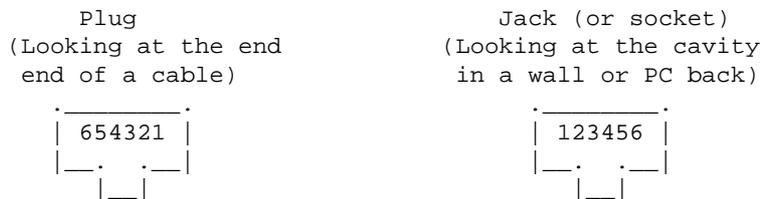
A standard MMJ null-modem cable has a MMJ connector at each end. It connects to the PC using a MMJ-to-DB adapter. This adapter plugs into a DB (say 25 pin) connector on the back of the PC and the MMJ connector plugs into it. If you don't have such an adapter, you can make a custom cable with a MMJ (or filed RJ) connector on one end and a DB connector on the other end.
