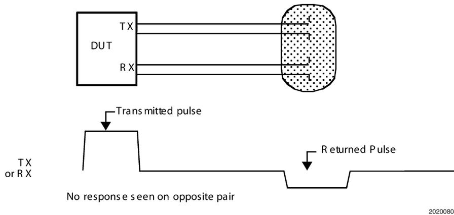
**FIGURE 4. Short Circuit Within a Single Pair**
