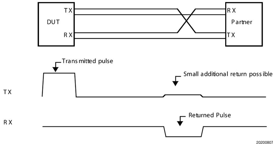
FIGURE 7. TX+/RX+ Cross-wired Circuit (into inactive or unpowered partner)
