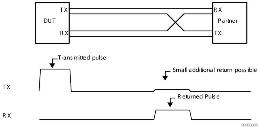
FIGURE 6. TX-/RX+ Cross-wired Circuit (into inactive or unpowered partner)
